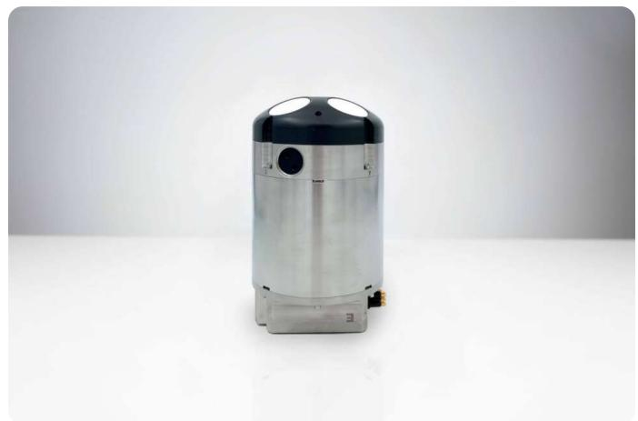
The DVL 1000 is our smallest survey-grade Doppler Velocity Log. It combines compact design with unprecedented functionality, being able to fly higher in the water column and closer to the seabed than similar equipment. It has a maximum operational depth of 6000 m and is ideally suited for subsea navigation where size and weight are a concern. This 1 MHz Doppler Velocity Log is used by industry leaders in the subsea market because of its high accuracy and state-of-the-art technology.
