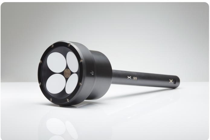
The DVL 333 Surface is a Doppler Velocity Log designed specifically for surface vessels. Traditional DVLs have a more vulnerable protruding head. The DVL 333 Surface mounts flush to the vehicle hull, alleviating this concern and minimizing drag and the risk of cavitation at the head.
